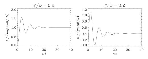
Critically-damped driven oscillator:
