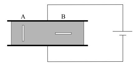
2. A solenoid is filled with a linear magnetic material of constant permeability  $\mu > \mu_0$ , which has two small cracks in it as shown in the figure. In which of the two cracks (A or B) is the magnetic field strength greater? Briefly explain your answer.
