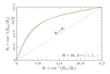
Note that  $\theta_2 > \theta_1$  for  $\theta_1 \in (0, \pi/2)$ , indicating that the downstream magnetic field is canted upwards towards the shock interface in an oblique fast-mode shock. This makes physical sense: a super-Alfvénic shock can sweep up the tangential component of the magnetic field and compress it without the field having time to rarify to produce a magneto-sonic wave, thereby driving the orientation of the magnetic field towards the shock interface.
