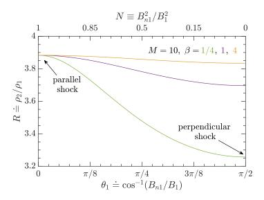
As expected (see (VIII.2.37)), the value of R decreases as the shock goes from parallel to perpendicular. Here is the angle  $\theta_2 \doteq \cos^{-1}(B_{n2}/B_2)$  that the downstream magnetic field makes with respect to the shock normal:
