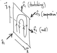
Any other configuration means that each time you stretch, you also compress – then antiparallel field lines are brought together and  $B^2$  decays resistively.<sup>31</sup>
