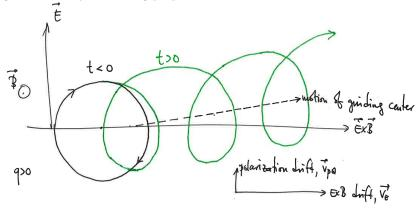
Because the ions and electrons have different signs of polarization drift, there is a current produced:
