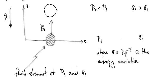
Displace flind element upwards while conserving its entropy. Now it has less entropy than its surroundings. With pressure balance holding, this means that it is also denser than its surroundings. It must fall back to its equilibrium position. Overshooting, it will oscillate at frequency N. (Mathematically, Do=0 → Dp/p=8 Dp/p → E-5hp= 75+85-5hp → f=1252.)
