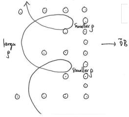
The grad-B drift is also charge dependent.
