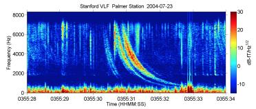
Because  $\omega \propto k^2$  implies a phase velocity  $\propto k$ , the highest-wavenumber/frequency waves arrive first, leading to the descending tone. Such observations can be used to measure the electron density of the ionosphere.
