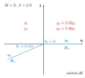
Solutions also allow for the reverse of this situation, called a 'switch-on shock.' In this case, a fluid with neither magnetic field nor flow velocity tangential to the shock front nevertheless acquires tangential components downstream of the shock, i.e.,  $B_{t2}$ ,  $u_{t2} \neq 0$  even though  $B_{t1}$ ,  $u_{t1} = 0$ . With T = 0 (N = 1), the momentum and induction equations provide
