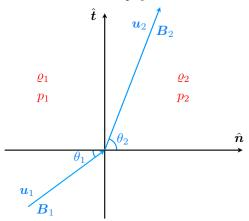
Equation (VIII.2.6) states that whatever mass flows into the shock must exit the shock in steady state:
