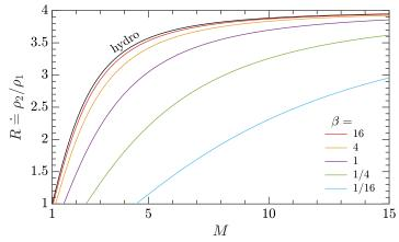
Stronger magnetic fields perpendicular to the shock normal reduce the compression ratio from its hydrodynamic value, while increasing the threshold Mach number for the shock to form.
