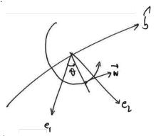
The coordinates  $(\hat{e}_1, \hat{e}_2, \hat{b})$  are functions of (t, r) as the particle sweeps around the changing, inhomogeneous magnetic field. What follows is a gradual shift of the particle coordinates from (r, v) to  $(R, v_{\parallel}, w_{\perp}, \vartheta)$ .
