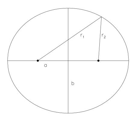
Ellipse with e=0.5. a and b are the semi-major and semi-minor axes, and the foci are marked by dots
