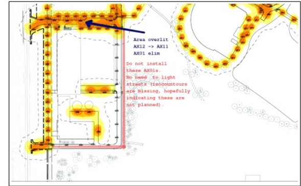
Fig. 29: Suggested changes to the current lighting plan. I assume all AX01 fixtures with no light contour would not be installed. The suggestion is to eliminate all AX01 fixtures except those 5 in the bottom right corner that may be around parking areas.
