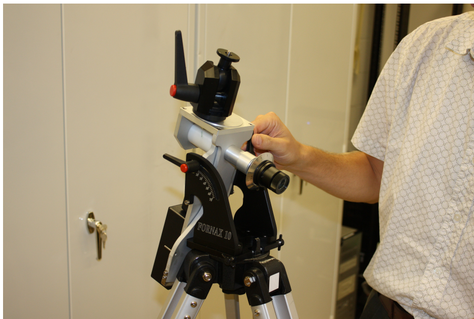
Figure 10: There are two locks on the altitude (up/down tilt) adjustment , on on either side. The professor is holding one of them. Unlock by turning counterclockwise (they may be stiff). You can move the handles out of the way by raising them and then rotating (think of this as pushing the red button, but instead of it going in, the rest of the handle lifts up). Princeton has a latitude of about 40^{\circ}20' N, so the North Star appears at about 40^{\circ}20' above the horizon. If the top of the tripod is horizontal (which is rarely the case), one would set the mount's altitude to 40 degrees. In practice, you need to perform this so-called polar alignment by looking through the polar axis or polar telescope.
