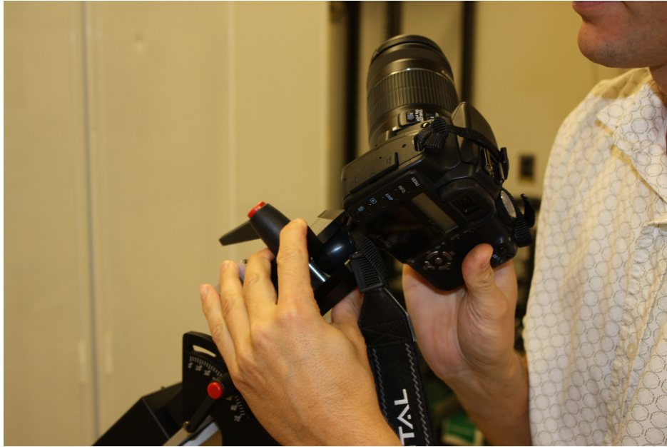
Figure 17: Readjust the joint to aim at whatever you like. Remember, this is the only way to aim. If you move the tripod or change the mount orientation, you will have to redo the polar alignment. So try to avoid “kicking” in the tripod, or moving its legs in any way.
