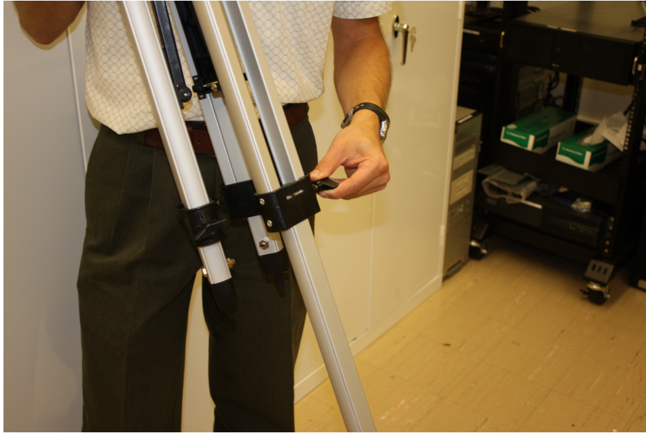
Figure 3: Extend the leg, and then tighten it by turning the knob clockwise. Make absolutely sure that the screws are tight.
