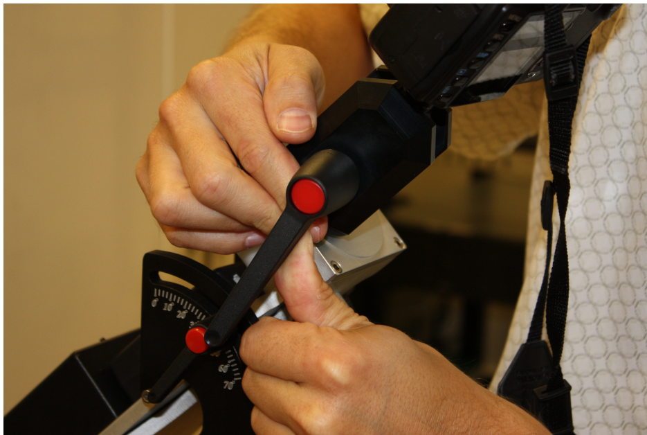
Figure 18: If it is in the way, you can rotate the latch to a different position by lifting it away from the tripod and turning it. Think of this as pushing the large red button in the middle of the latch, but instead of the button depressing, the latch will raise up. You can then turn it without loosening the joint.
