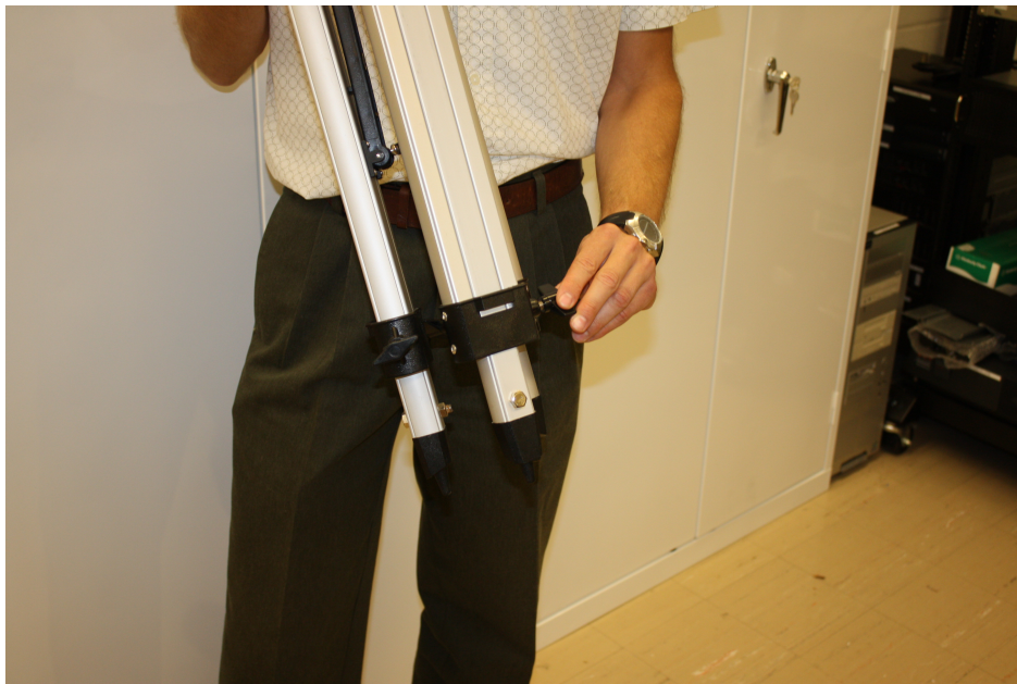
Figure 2: At the bottom of each leg there is a knob. Twist this counterclockwise to loosen the extension .
