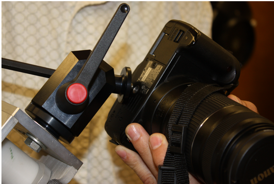
Figure 15: Attach the camera by screwing the bolt into the bottom of the camera. Make sure this connection is secure.
