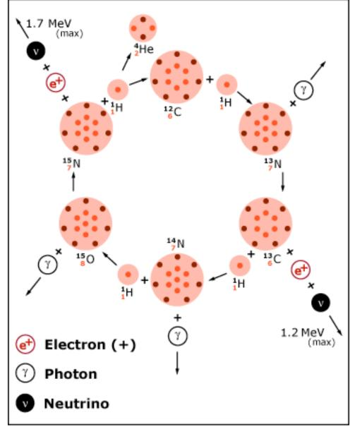
Uses C, N, and O nuclei to catalyze fusion of H into He
