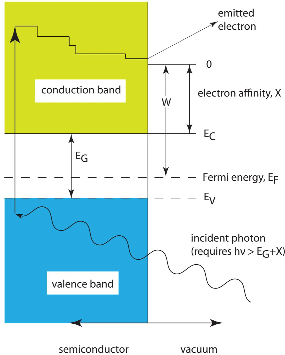
Photoelectric effect in a semi-conductor (energy band diagram)
