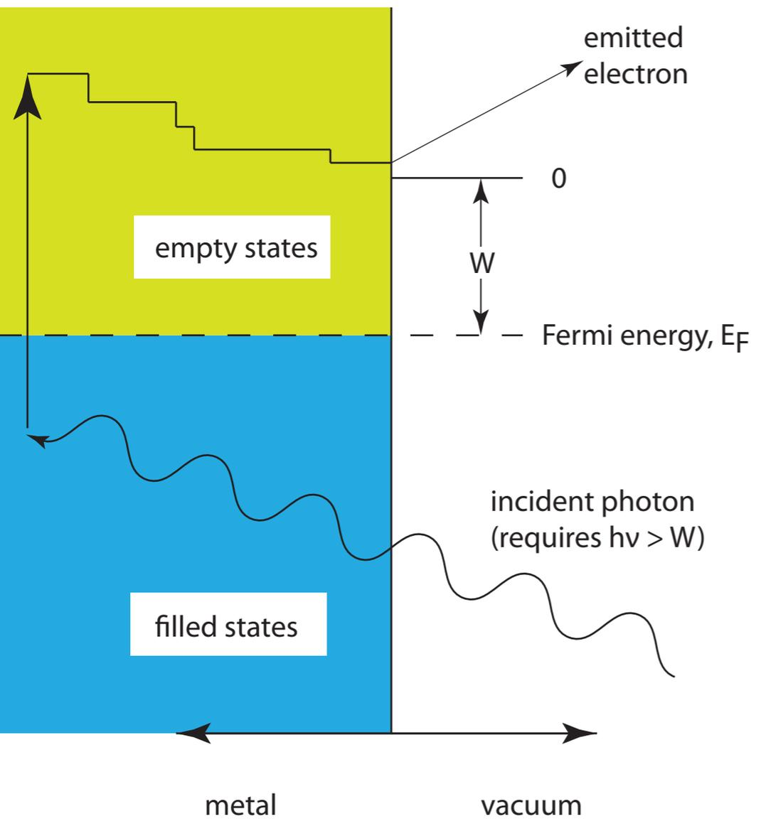
Photoelectric effect in a metal (energy band diagram)
