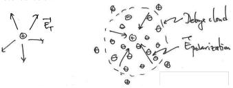
Note that the electric field due to the polarization of the plasma in response to the ion's bare Coulomb potential acts in the opposite direction to the unshielded electric field.
