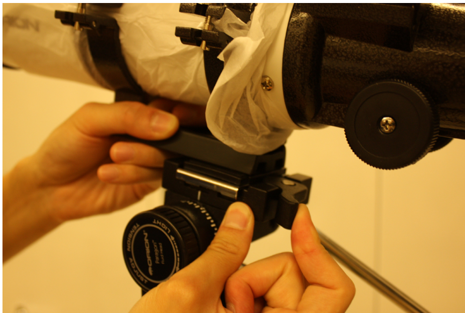
Figure 9: Mounting telescope step 3: Snap the lever shut. Ensure the telescope is securely mounted on the tripod.
