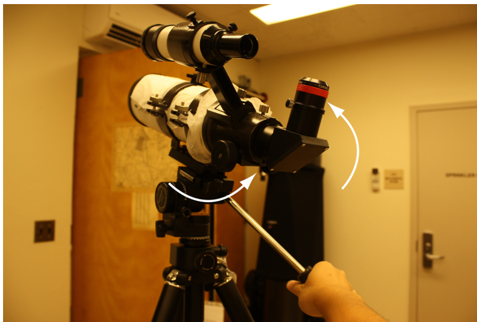
Figure 17: You should now be able to move the telescope freely in both axes.
