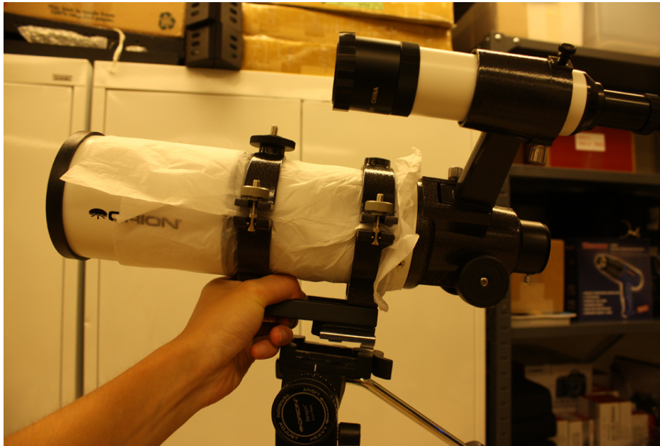
Figure 6: The telescope mounts onto the tripod in this direction. More detail in the next three points. Caution: You may find this a two person job at first.
