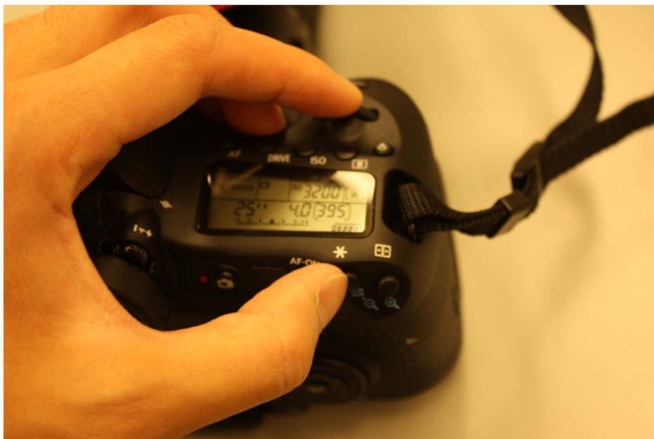
Figure 19: To change the focal ratio, press the '*' button and twist the dial at the same time. A smaller focal ratio gives a wider aperture, and allows more light to get through. We usually use the smallest focal ratio available.
