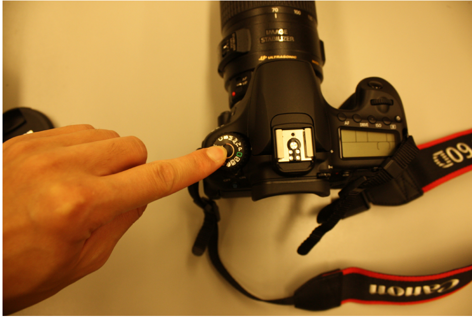
Figure 7: To change the exposure mode, press on the central button, and then twist the knob. During day time testing, we will change the mode to P for 'Programmed Auto'.
