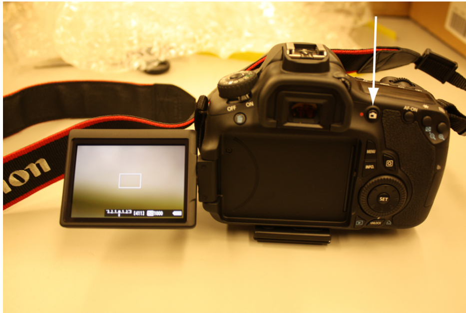
Figure 15: To access live-view, press here. This turns the camera into a video camera, and is very useful for focusing. Try to focus using live-view on a very bright star
