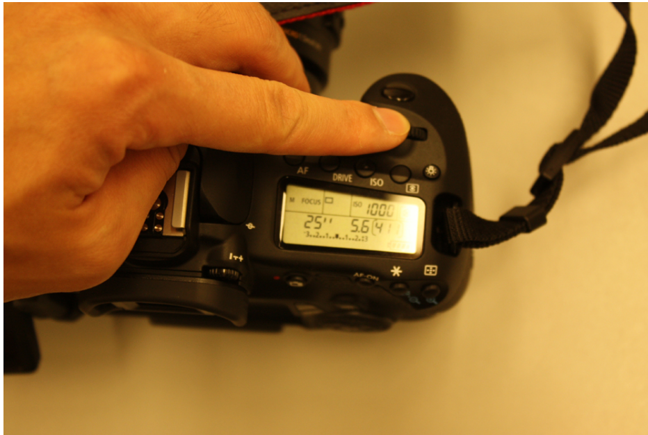
Figure 17: Change the exposure time by twisting this dial. For the moon, an exposure time of a fraction of a second is fine. To take images of stars, exposure times should be around 30 seconds (30"). A longer exposure time gathers more light, but is more demanding on an accurate polar alignment and dark sky background. Try different exposure times to see what works best for the conditions. You can also choose the B setting to have an indefinite exposure time.
