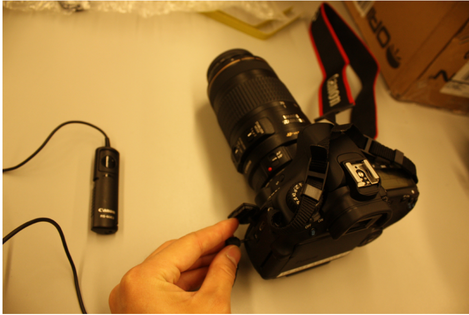
Figure 11: Connect the remote shutter control. During night time, we will use the remote control to take images. This prevents camera movement when the shutter is pressed.
