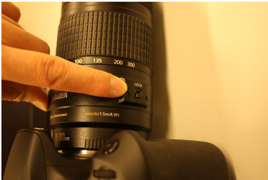
Figure 6: Set up the lens for astronomy images: 3) Unlock the lens so we can change zoom and focus.
