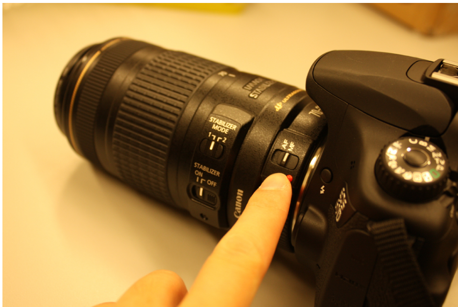
Figure 4: Set up the lens for astronomy images: 1) Change to manual focus - there is not enough light for autofocus to work.
