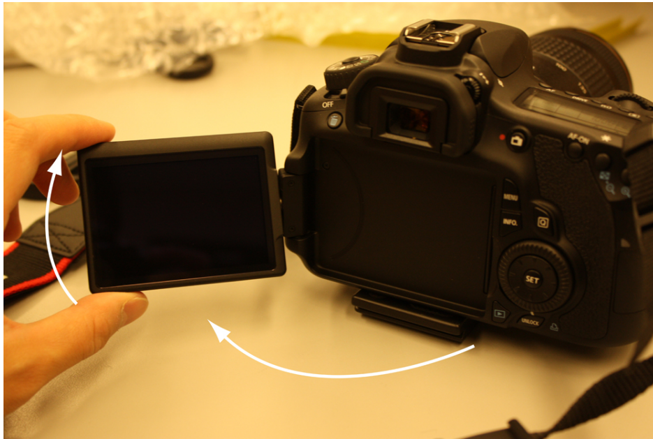
Figure 13: You can open the display to view the image, or to use live view
