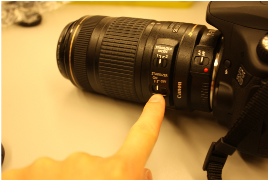
Figure 5: Set up the lens for astronomy images: 2) Turn off image stabilisation, since we will be using a tripod.
