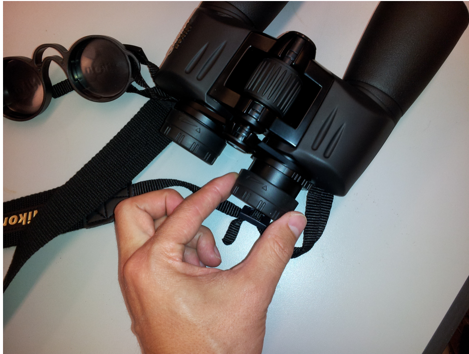
Figure 4: Twist the ring at the end of each eyepiece to adjust how much it overhangs the lens.
