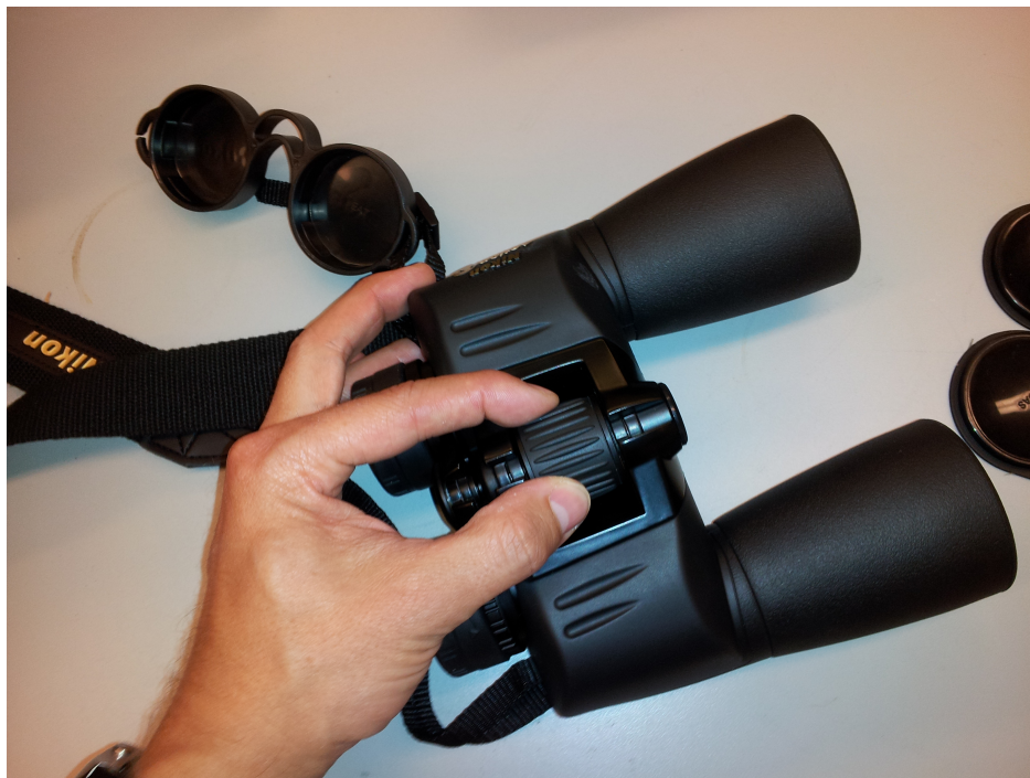
Figure 5: The focus can be adjusted with the dial in the middle. Adjust it so that your left eye sees the sharpest image. If you have contacts you can keep them in, but if you have glasses you should remove them and leave the vision correction to the binoculars. Remember that the proper focus depends on the distance to the object, so if you are going to be looking at stars and planets “at infinity,” you should be looking at such objects when you focus.
