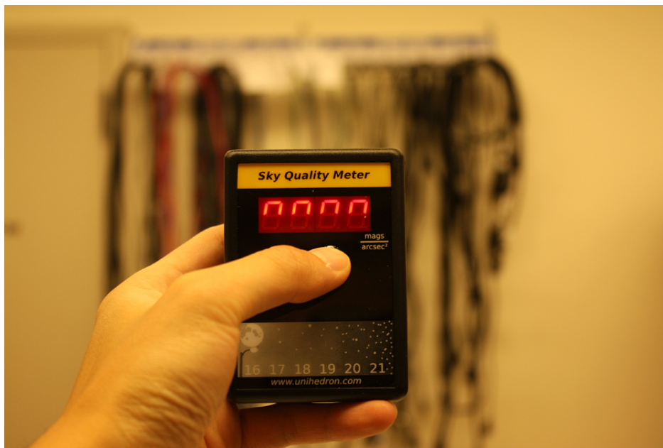
Figure 3: In some cases, the sensor may be saturated and unable to provide a proper reading (see picture). This can happen if the sensor is being tested during daytime or indoors.
