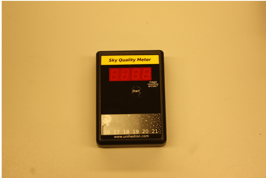
Figure 1: The Sky Quality Meter measures the sky brightness in units of magnitudes per sq arcsecond.
