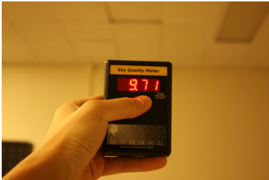
Figure 2: To use, find a place with no direct illumination from nearby street lamp, car headlights, etc. Press the start button and record the reading. A value of 16-18 mag/arcsec 2 is expected under city skies, whilst the darkest skies are at \sim 21 mag/arcsec 2 .
