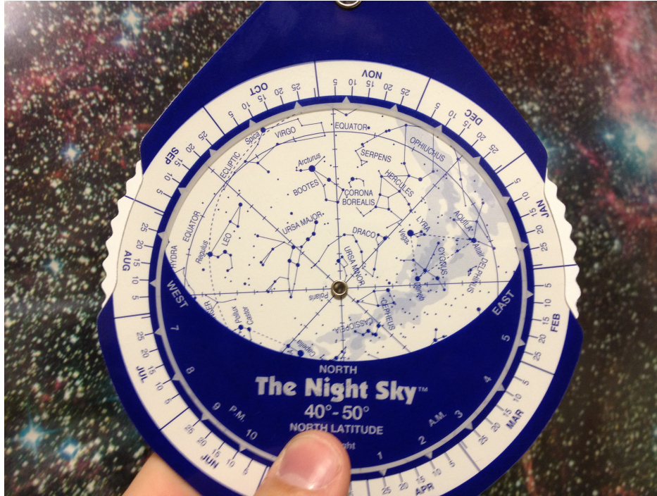
Figure 3: Once the wheel is set, locate Polaris and align the center of the Planisphere with it. This side will show you the sky to the North, with the blue border representing the horizon. To locate Polaris, find Ursa Major (the Big Dipper ) and follow the line of the two stars at the outside of the bowl.
